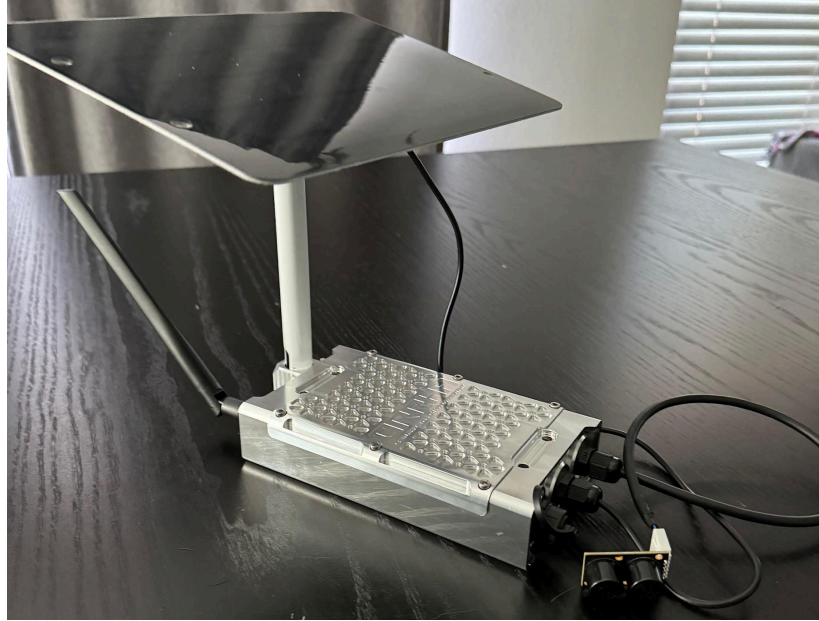
Figure 15. Aluminum Milled Sensor Node Housing
