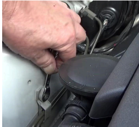
Release pipe clamp (allows booster to move)
