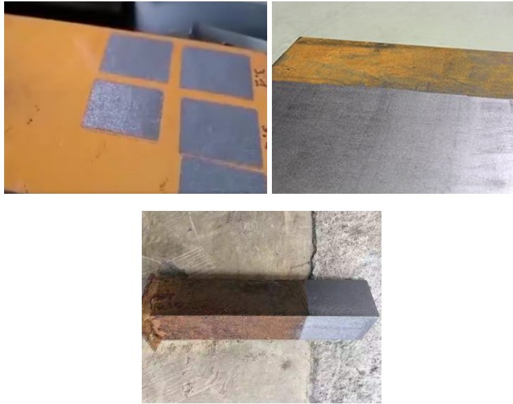
d laser rust removal Figure 2.2 Typical laser cleaning applications
