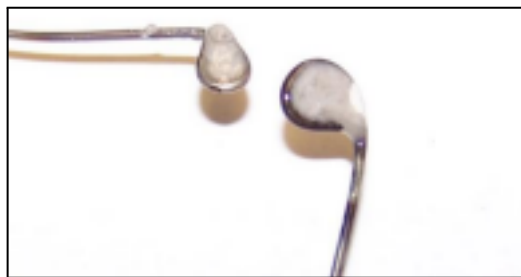
Figure 6. Beads that have a gray, milky color rather than a transparent, bright color due to the gas bubbles that remain trapped in the amorphous borax.
