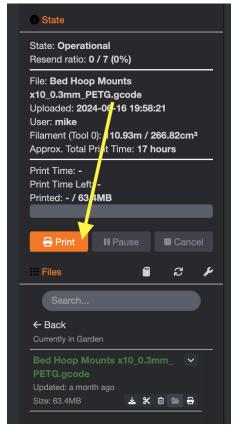
**Make sure the printer is ready** - correct filament type and color loaded, bed prepared, etc. When ready, click "Print" to start!
