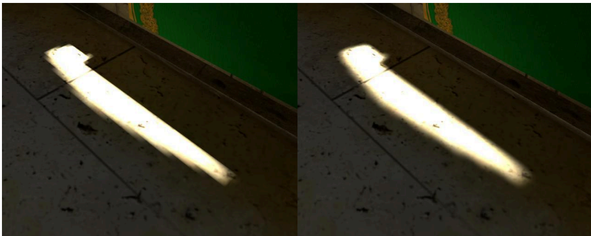
Left: default bilinear filtering. Right: bicubic filtering.
