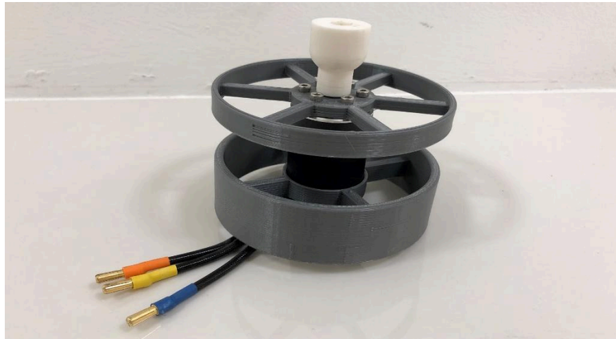
A7: Assembled Motor, Spindles and Adaptor
