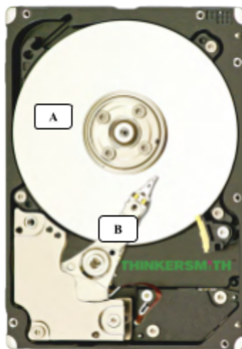
A) Spinning Storage Platter B) Read/Write Head
