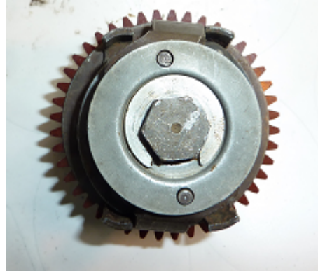
20. Fit the dished washer and 'C' washer
