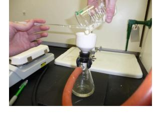
flask containing the liquid on the hotplate and slowly boil away the acetone:ether mixture. You may find that maintaining a vacuum greatly speeds this process. Why?
