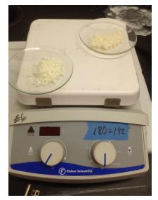
3. After allowing ten to twenty minutes for any remaining solvent to evaporate, weigh.
