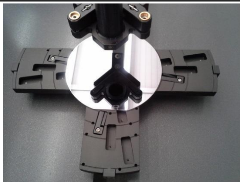
Figure 4 A bare Si wafer on the stage for baseline measurement.
