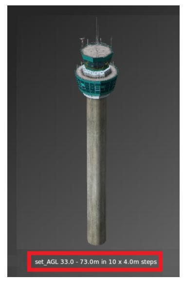
For an adjustable tower model, the available height options are shown at the bottom of the preview pane. This is expressed as a minimum and maximum height range, with the correct increments to use for this specific model.
