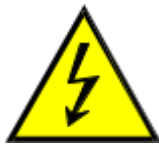
Figure 1 Marking of high voltage equipment
