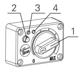
The controller contains rotating dial, button and two indicators:
