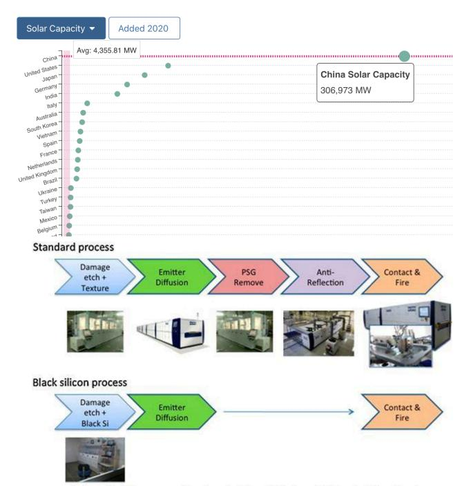
Schematic of the process flow for a traditional SiNx based AR coated Si cell and a b-Si equivalent.
