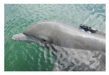
Photo - Dolphin With Tag: A dolphin wearing a biologging tag. The tag is attached to the animal using suction cups, and can measure the sounds the animal hears, sound the animal uses to communicate and echolocate, as well as the motion of the animal. Credit: Alex Shorter, University of Michigan
