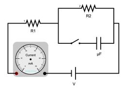
Step 2: Fill in the voltage of the battery and the capacitance of the capacitor. Then use arrows to show the flow of electricity through the circuit while the switch is first closed and the capacitor is still uncharged as shown below. Also show the location of the needle when the switch is first closed. Calculate the value of R1 and then determine R2
