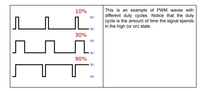
PWMs are often used to transfer average power. For example if you have a 5V pin and you send a PWM signal with a 20% duty cycle it would transfer an effective one volt across the line. If you run a 5v line with a 100% PWM you would get the full 5v transferred across the line. This technique can be used for running motors faster or slower and for dimming LEDs by providing average power over time. See the code snippets below for how to use the PWM APIs.
