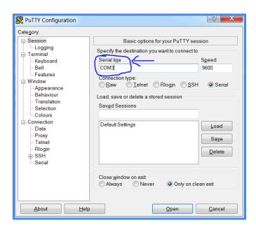
4. Check the **Speed** parameter. All mbed microcontrollers default to 9600, and this is also the default on PuTTY, so you shouldn't have to edit this parameter.
