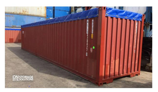
Open-top containers are designed for cargo that is too large or awkwardly shaped to be loaded through standard doors. Cargo is loaded from above using cranes. They are available in standard sizes like 20ft and 40ft. A 40ft open-top container has internal dimensions of approximately 12.03m in length, 2.4m in width, and 2.34m in height.
