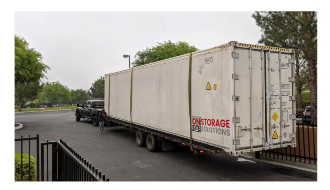
Refrigerated containers, or reefers, maintain a controlled temperature for perishable goods. They come fitted with cooling systems and thermal-resistant walls. Common sizes include 20ft and 40ft, with a 40ft reefer having internal dimensions of approximately 11.56m in length, 2.28m in width, and 2.25m in height. Reefers can maintain temperatures ranging from -30°C to +30°C.
