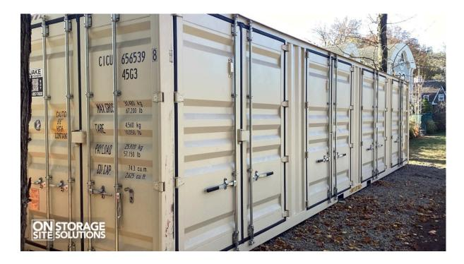
Side-opening containers feature doors that open along the long side of the container, making access easier. They are useful for loading and unloading specific pallets of goods and are available in both 20ft and 40ft variants.
