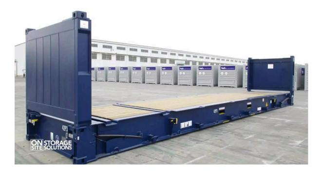
Flat rack containers have collapsible sides and are suited for heavy or oversized cargo. These containers essentially lack sidewalls and a roof, allowing for easy loading of large items. They are commonly used for items like heavy machinery, construction materials, or oversized vehicles. A 40-foot flat rack container is often used for oversized cargo that doesn't fit in a regular container.
