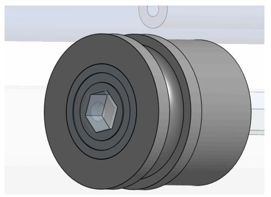
5. First, loop the other side of the 135T belt onto the pulley that is not smooth. Next take your threaded hex shaft stock, and fit it through your hex shaft, and leave it at the end. Take a 10-32 bolt, and thread it through the tapped hex-shaft and the plate
