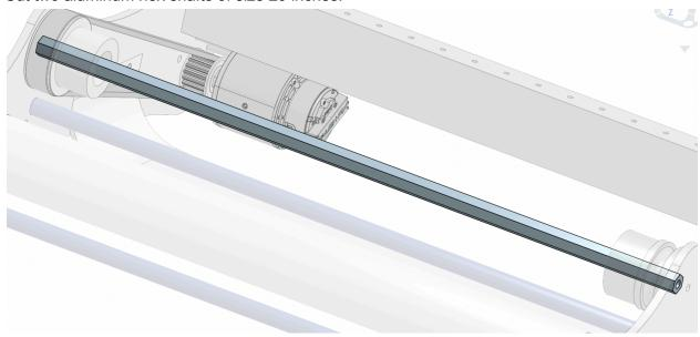
For the hex shaft, make sure to tap them with self-tapping bolts to an appropriate length for a 10-32 fastener to fit through.
