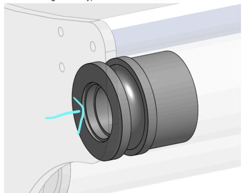
Print two pulleys, with bearing side facing up. Part id is : 5026-23-I03-PLApulley
