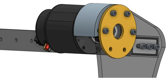
4. Put your bearing into the pulleys, making sure that it has a relatively tight fit. Repeat for all 4 pulleys
