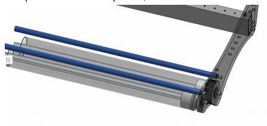
8. Take the o-ring, turn it into a figure 8 then attach onto the following pulley. Consult Neel/Mentor before doing so.
