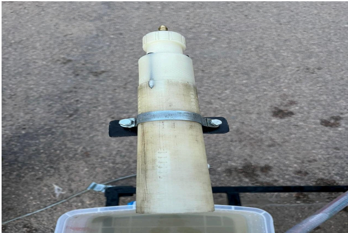
Figure: 3.11 Jet Pump2 (air and water)
