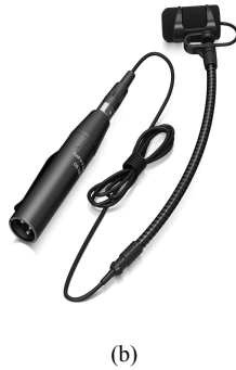
Fig. 1. Physical system separated into four major subsystems (a) overall system. (b) Behringer CB100 Gooseneck Condenser Microphone that records the flute and background audio and can be plugged into a laptop.
