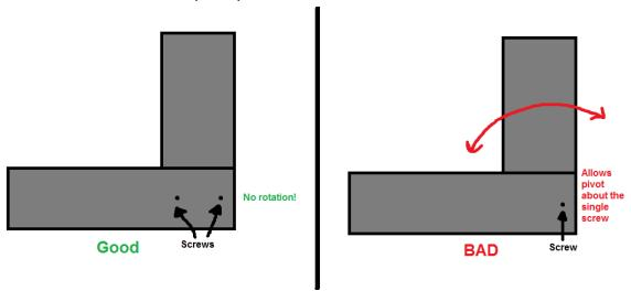
2.3.4.3. All axles need to be supported in at least TWO places. This refers to the stationary points in relation to the axle. (Not anything attached to the axle i.e. a wheel or a sprocket) Ideally these places are on opposite sides of the main load.
