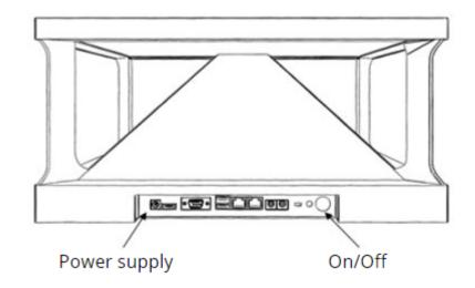
Start the Prism with the ignition button on the back of the product, and wait until charging is complete. To stop it, turn it off by pressing the same button.
