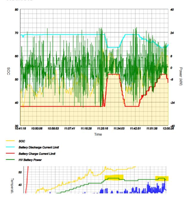
The top graph shows the battery charge and discharge limits. The second partial graph (of which the full one is below) shows the hybrid battery temperature in green with the yellow highlight showing the section we're interested in. This matches up with the first graph on time.
