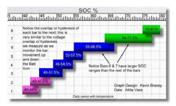
It's important to note that once the force recharging process begins it will forcibly charge the battery until it reaches 47-50% (4 bars), which takes around 2-3 minutes. The only time the engine will shut off during this is if you shut the car off yourself.
