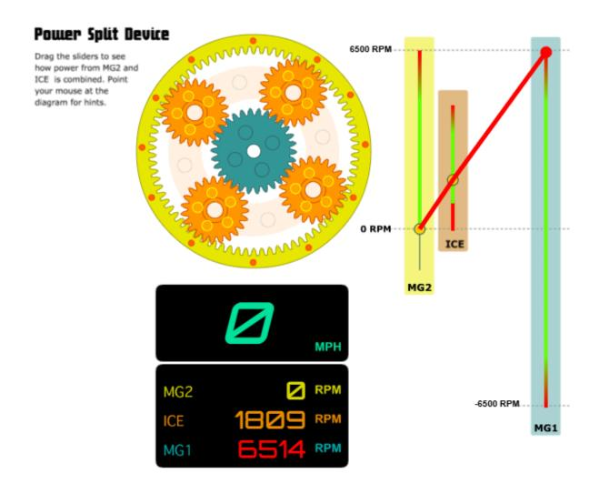
When at a standstill and the RPM of the engine increases, MG1 must spin faster to counteract the effect of the engine's RPM increasing. It has to do this because if it didn't then this would mean a transfer of torque through the planetary gearset to the wheels (MG2) and this isn't always desirable (such as when in park or coasting).
