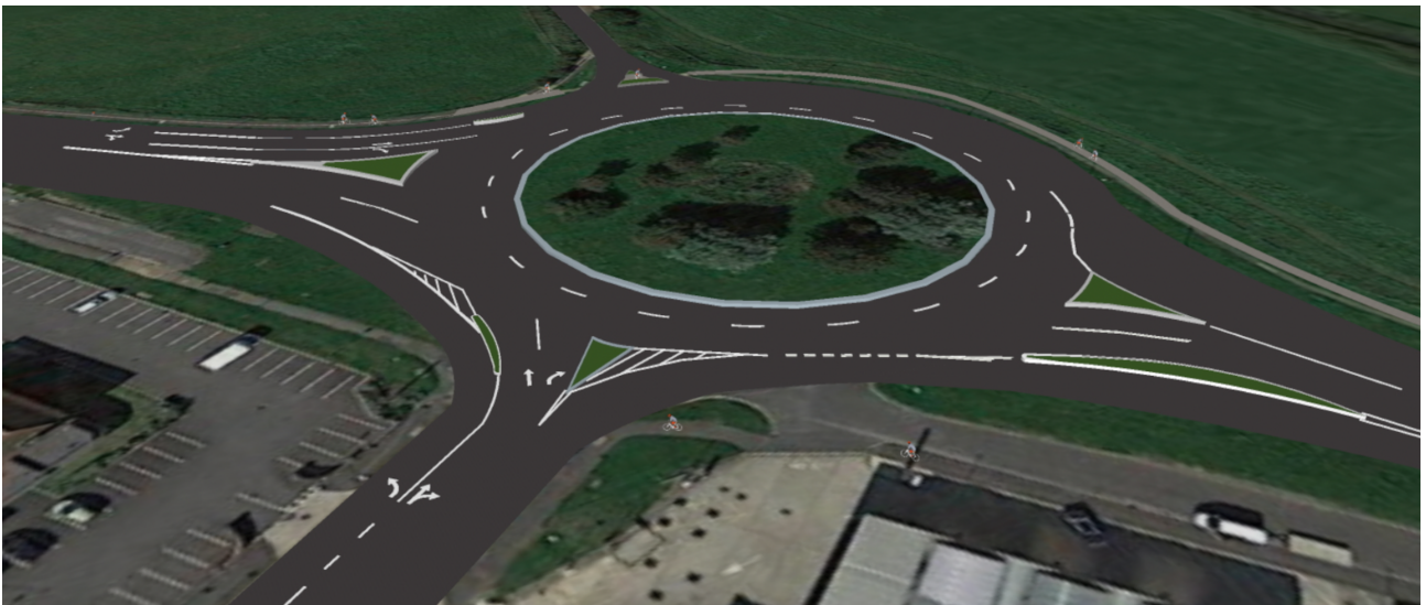
Concept B: Increased road-width, improvements to road markings, dedicated lanes and traffic-merging lanes lanes.
