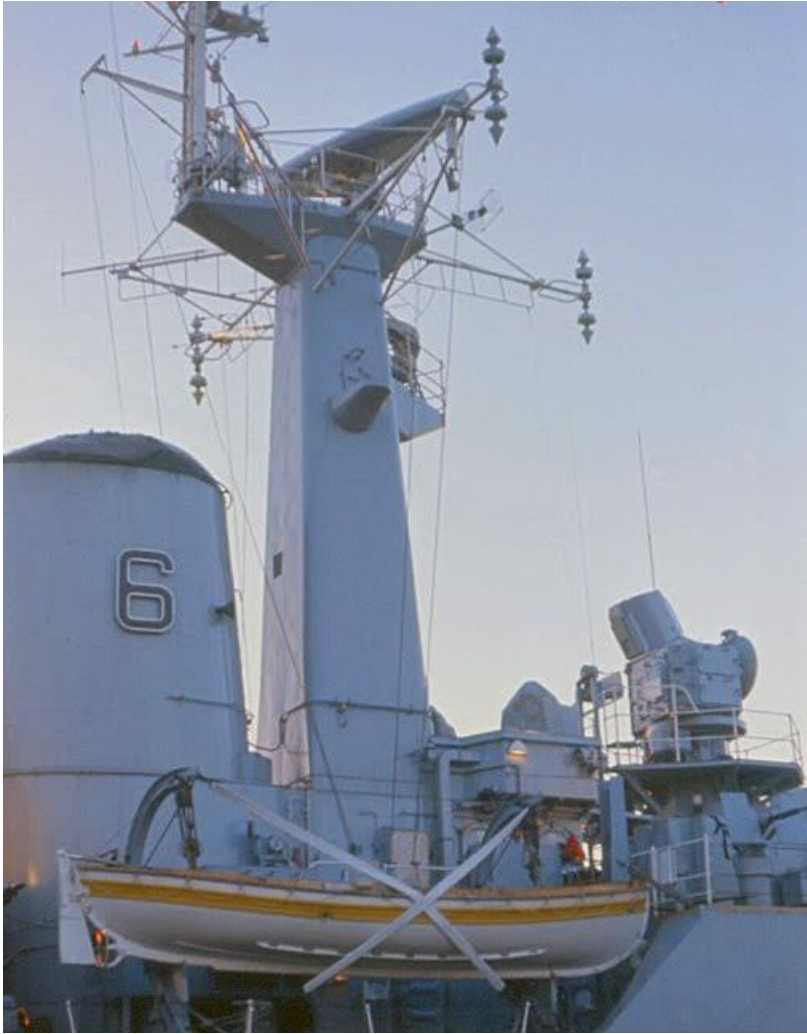
Type 12 Frigate (HMS Plymouth and HMS Yarmouth) detail. Note 'cheese' antennae of 993 radar on foremast for air warning, Type 903 fire control radar above bridge, and to the right, a 20mm 7A Oerlikon gun.
