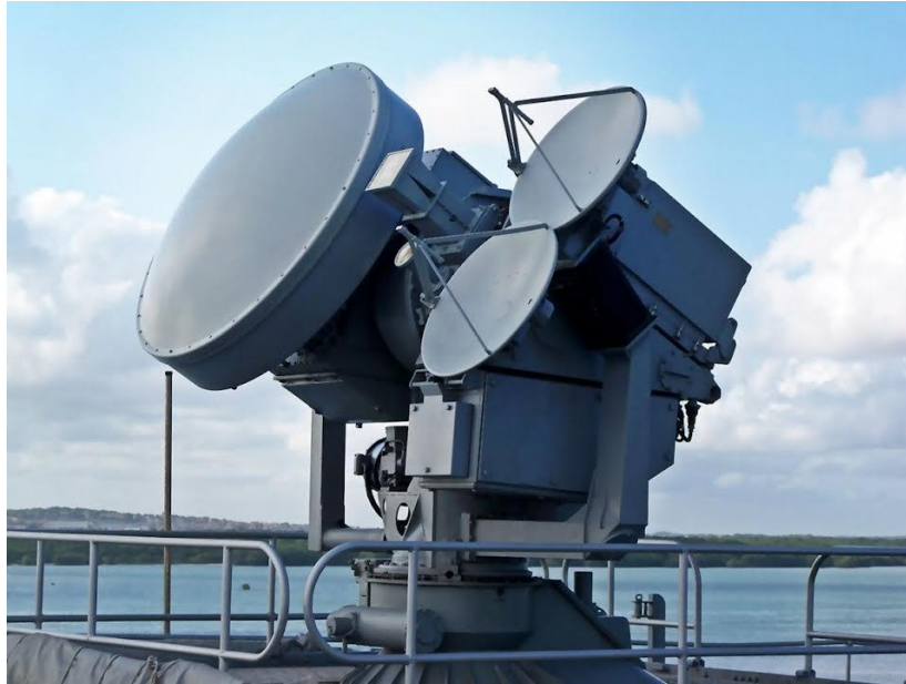
Type 910 radar for SeaWolf, as fitted to HMS Broadsword and HMS Brilliant
