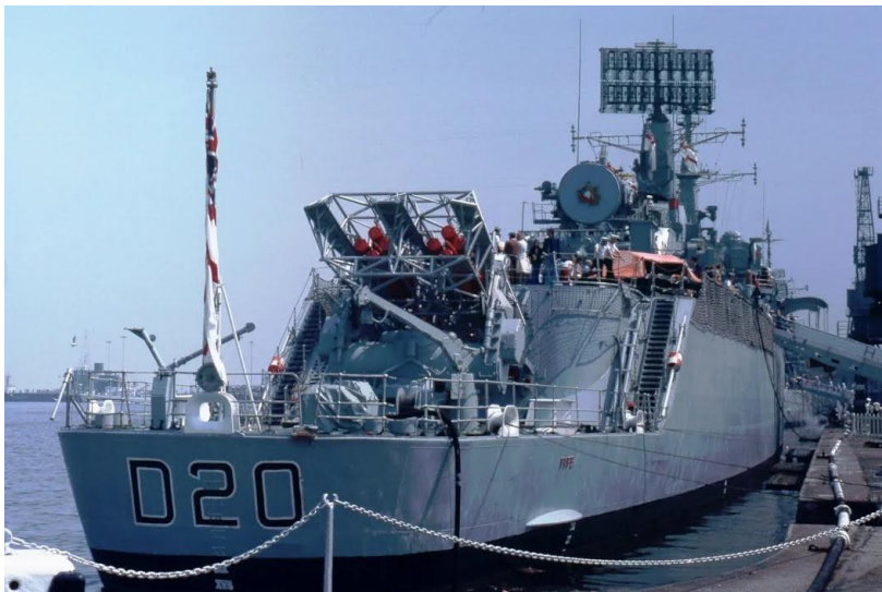
SeaSlug missile launcher with large dish of the Type 901 fire control radar above the hanger on County Class destroyer
