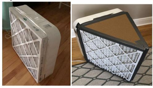
These improvised fans can be quite effective, one tested by <u>CBC Marketplace</u> produced a Clean Air Delivery Rate (CADR) of 100 CFM, in line with commercial filters that cost hundreds of dollars.
