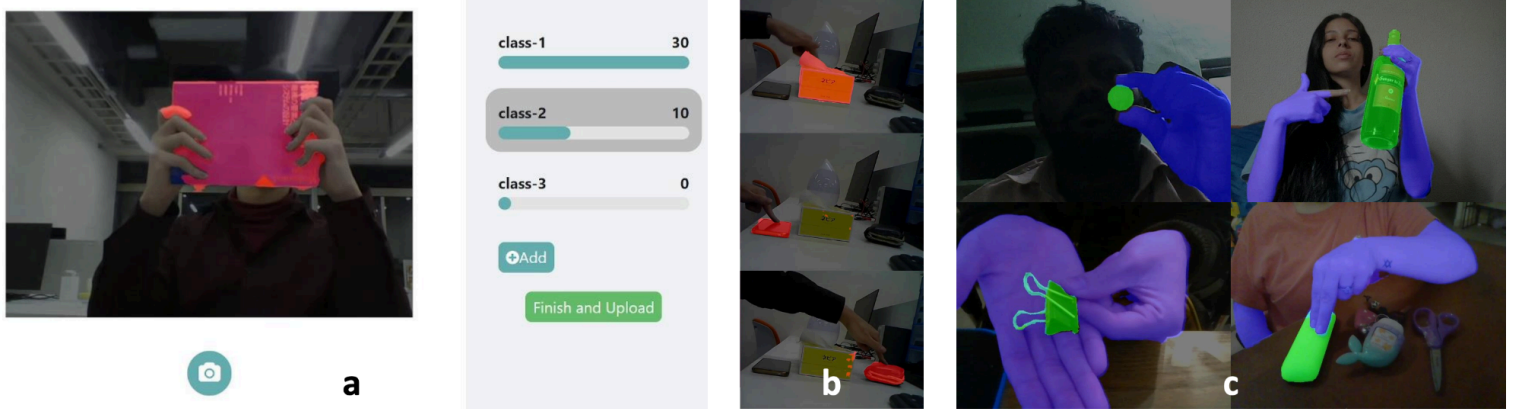
Figure 1: (a): The teaching interface of our vision-based Interactive Machine Teaching system, LookHere. LookHere provides a segmentation mask (an object highlight) on the object guided by users' deictic gestures in real time during teaching. This segmentation mask is used for model training as additional information for training classifiers. (b): Users' deictic gestures guides in-situ object annotations. (c): Example images in our HuTics dataset that enables the implementation of LookHere. HuTics includes 2040 labeled images that capture how 170 people use deictic gestures to present an object.
