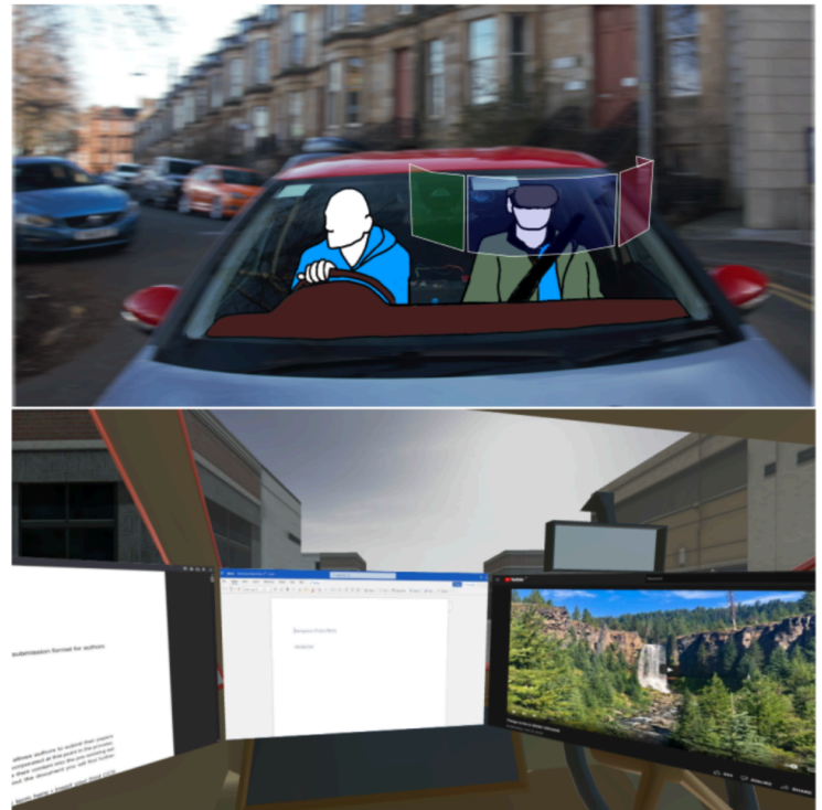
Figure 5: The Movement-Locked Content for Productivity application, where a single user interacts with web-based word processor, pdf and video content locked to the reference frame of the virtual vehicle they are sat inside. A digitised city route updates around the vehicle based on the real location.
