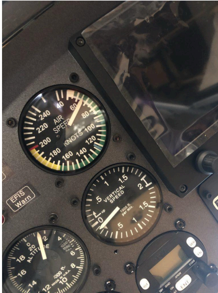
Photo 7-2 Analog instruments during Pitot check
