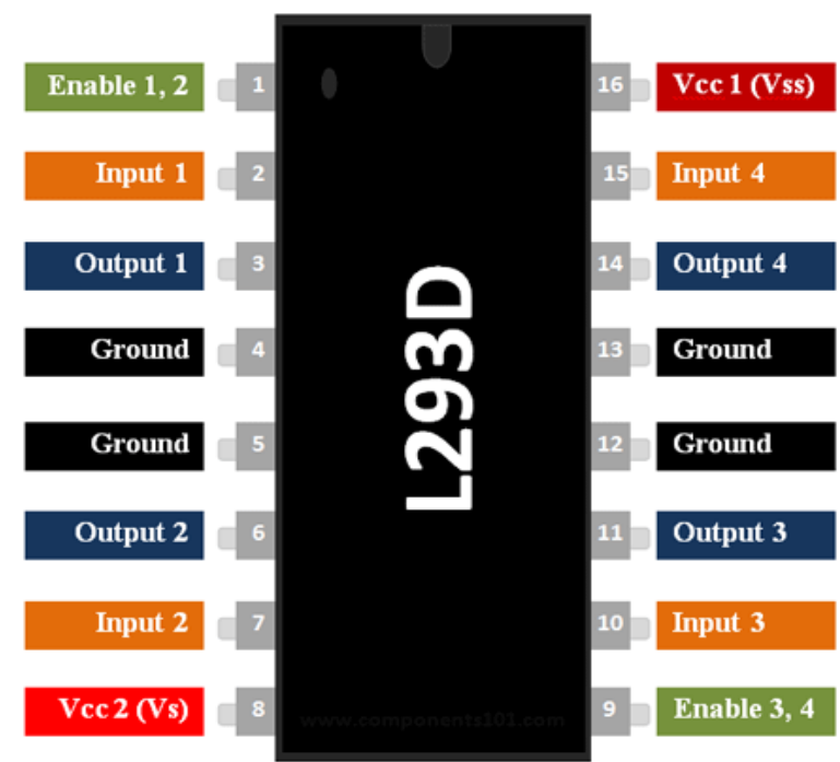
FIG 3.8 L293D Pin Configuration
