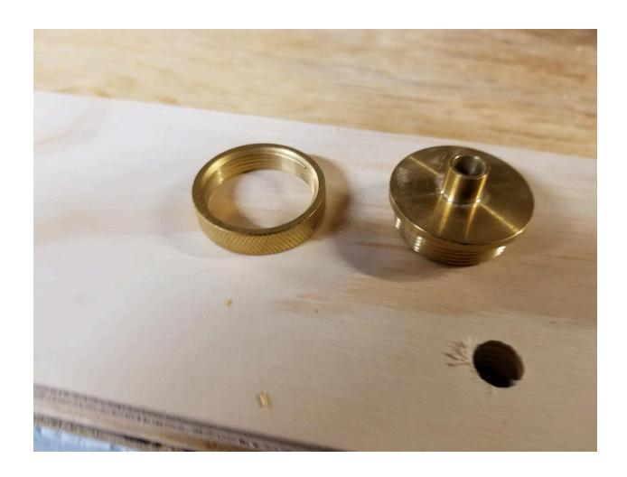
There are several styles of template collars, but if you use the kind we prefer, the part of the template with the collar is inserted into a recess in the router base-plate and the ring is screwed onto it.
