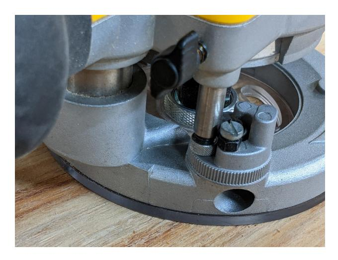
You're done with the setup so you can now release the locking lever so that the bit retracts. With the Depth stop set that way, the bit will cut  $\frac{3}{4}$ " deep (Red setting below) when it is plunged until the adjusting rod hits the stop. If you rotate the stop to the next tallest position the bit will cut  $\frac{1}{2}$ " deep (Yellow setting) and at the next tallest it will cut  $\frac{1}{4}$ " deep (Green setting).
