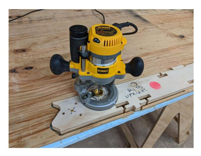
We use a DeWALT DW618 (above) for all the cutting with the  $\frac{1}{4}$ " bit, and a DeWALT DWP611 (below) trim router for drilling with the  $\frac{1}{8}$ " bit, but if necessary the Dewalt 611 can work for everything by using multiple shallow passes. The brand and size of tools is up to you, but as with all tools in most cases more power is better.
