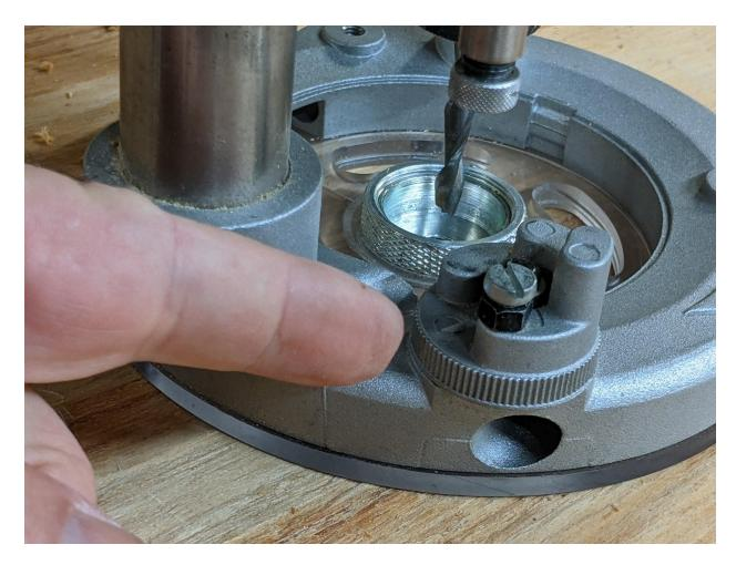
Loosen the locking nut on the adjusting rod and extend it until the end of the rod is firmly on the depth stop. Tighten the locking nut so that it's good and tight...you don't want anything to slip!
