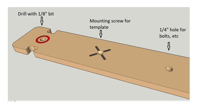
The rule of thumb is that if a hole has a **red circle** around it to drill with the ½" bit..it's a pilot hole for a screw. If it has a **black X** across it it's for holddown screws to attach the templates to the material. Feel free to reposition the holddown screws to anywhere that makes sense to you,
