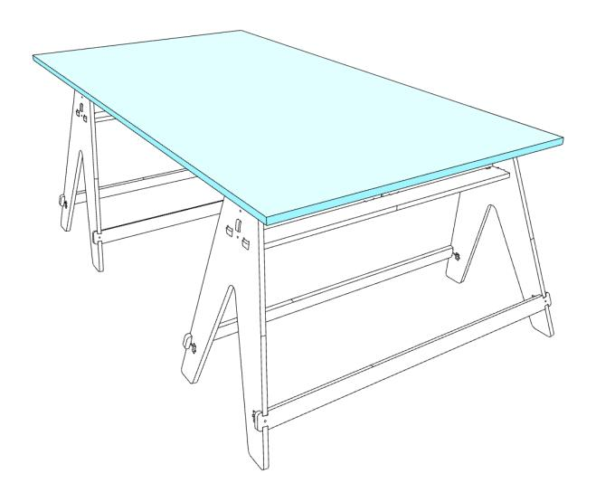
On top of this foam "spoilboard" you'll place the material you'll be cutting your Sheldon out of..the sheets of coroplast,  $\frac{1}{2}$ " plywood, and  $\frac{3}{4}$ " Advantech or plywood
