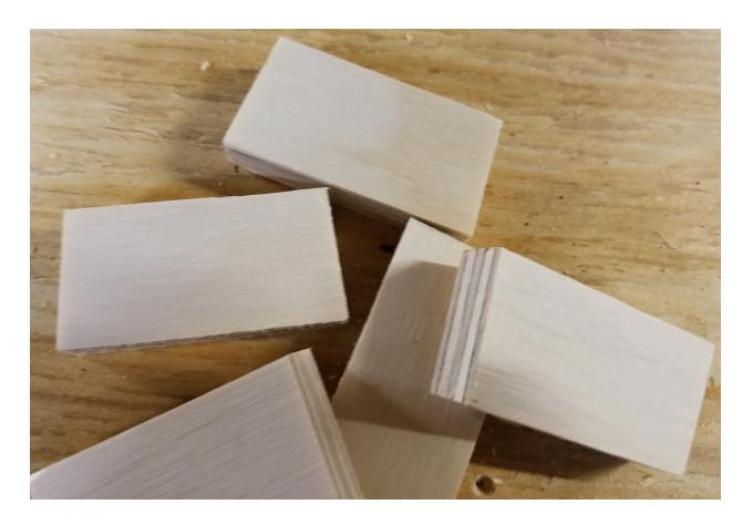
The keystone-shaped hatchets are the one part you can't sensibly cut "tradigitally" with templates, and unfortunately you'll need a lot of them...250+. Luckily there are a couple of options for fabricating them: cutting with a CNC machine or using a tablesaw or chopsaw:
