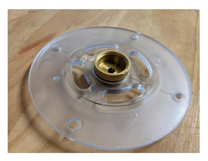
It's critical to get the ring REALLY tight so that it doesn't vibrate loose. A big pair of pliers on the rings will usually get it tight enough, but a dot of temporary thread locker like blue Locktite will make it secure but permanent. If you use thread locker you may have to replace the router's baseplate if you need to replace the collar, but it's a *REAL* hassle if the collar comes loose while you're cutting!
