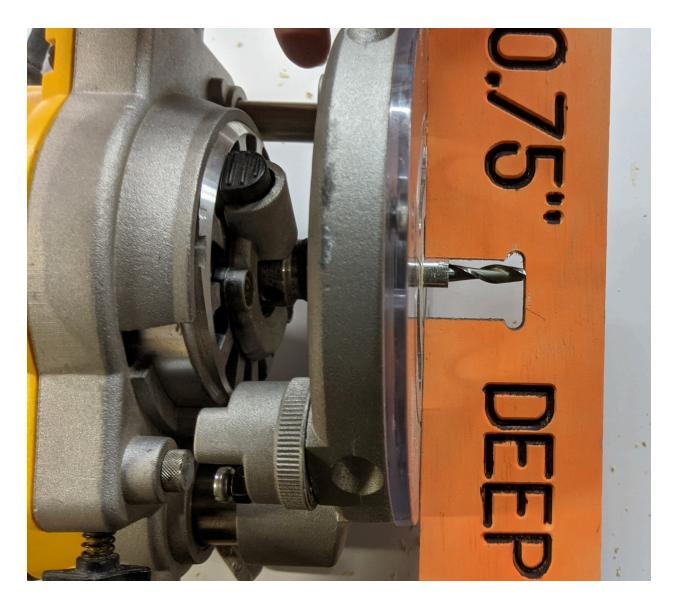
Lock the router at that depth using its looking lever and double-check the depth with the template. If it's not right keep messing with it until it is!
