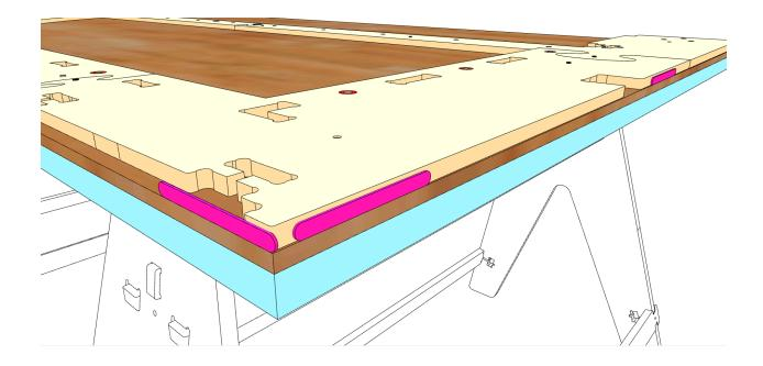
For some features like pockets and large holes where the sawdust can't easily be ejected by the bit, the sawdust will tend to pack in the corners and block the template collarand you'll need to stop occasionally to remove any dust that's accumulated. A ShopVac works great but you can also use an air compressor to blow the chips out. If you don't have either of these you can clean it out with your finger (after stopping and removing the router of course!).
