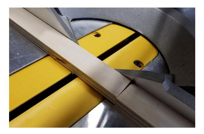
Trim one end of one of your 1" wide strips, flip it over, and cut the other end. Continue flipping and cutting until you have at least 250 hatchets. You'll have to check the first couple of them and adjust the fence to make sure they are the right length, but after that it's a simple process of cutting and flipping.
