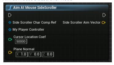
The Aim at Mouse SideScroller will take in a character component reference to see where it is in the world, your player controller to determine what the mouse cursor is, a cursor location coefficient to determine the depth and the plane normal for the plane normal.
