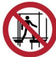
Do not use incomplete scaffold
