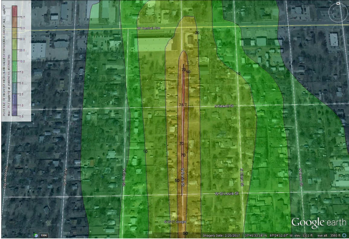
Figure 4 - AERMOD results showing 24-hour first highest PM10 concentrations in µg/m3, zoomed view of Figure 3
