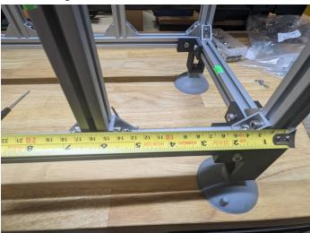
• Measuring from the outside edges ensure 185mm between the 200mm height beams:
