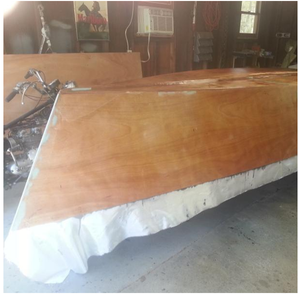
Fiberglassing The Hull
