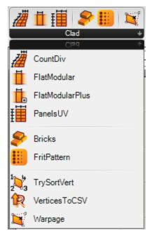
Cladding tools or "Clad" are components related to modeling building enclosures.
