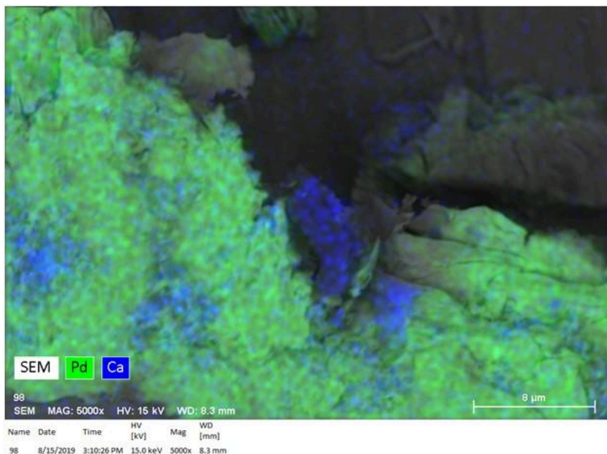
Image 7. Pd deposited by rubbing on the mesh, showing embedded \text{CaCO}_3
