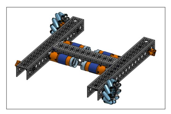
22. Repeat the process and attach the white mecanum wheels to the opposite corners of the chassis.
