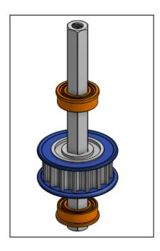
8. Secure the Hyper Hub to the top of the Axle. You will need to make four of these parts.
