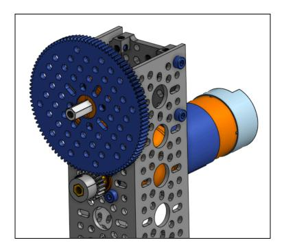
12. Attach the 17 hole shallow U channel to the 100 tooth gear.
