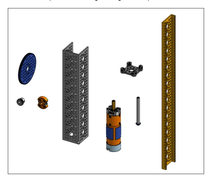
2. Place the Quad block on the top of the 10 Hole U Channel.
