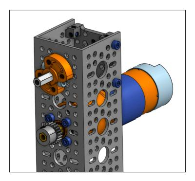
11. Attach the 100 tooth gear to the Sonic Hub.
