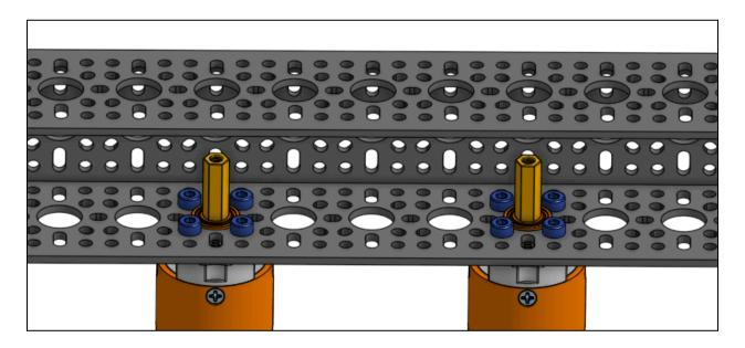
14. Attach an Axle assembly to the second hole from the end of the U Channel. You will need to disassemble the Axle assembly and then reassemble. Place a 55 or 64 tooth belt over the pulley before finalizing the assembly
