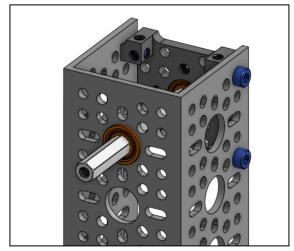
6. Attach the Sonic Hub to the end of the REV axle. In the example an offset of 1 inch on the Z axis was used.
