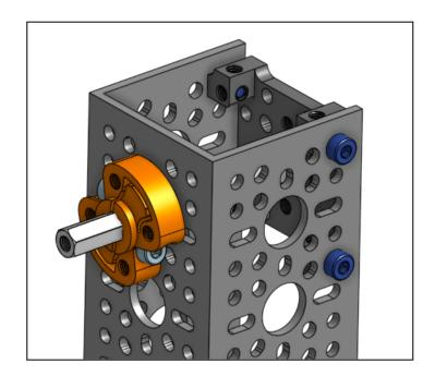
7. Attach the DC Motor to the third hole down from the top. Use the bolt opening on the DC motor and connect to bolt hole on the U channel for the best results.
