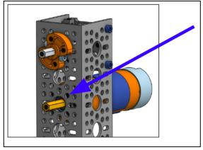
8. Attach the flanged bearing to the opening where the motor shaft extends out of the U channel.
