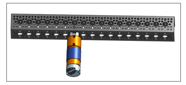
11. Repeat the process and attach the second DC motor 7 holes back from the other end of the U Channel.
