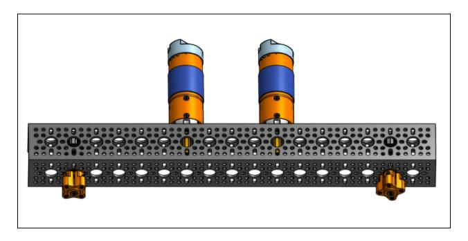
16. Attach two pulleys to the motors and tighten with the set screws using the 2.5mm Bolt Driver. (The belts are not shown below)
