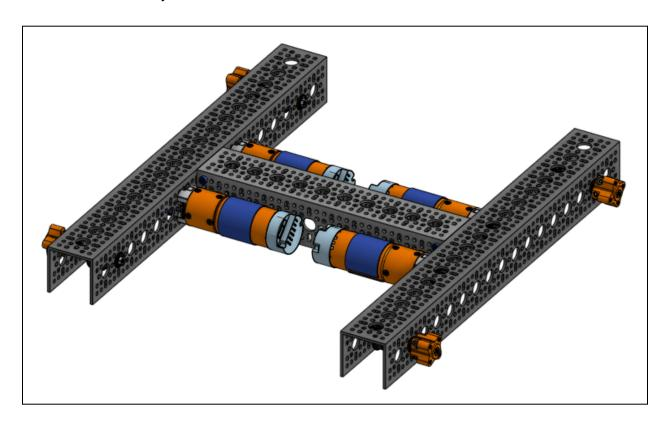
20. Use the 8x bolts and attach the Crossbeam Quad block to the Rails. (Both left and right side)
