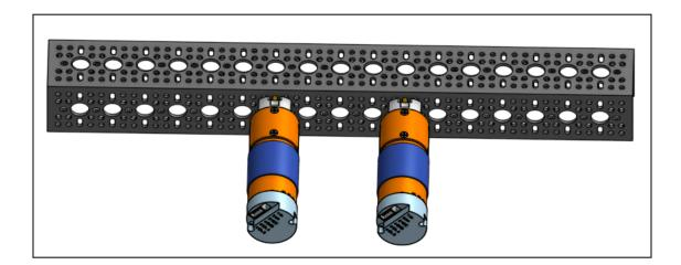
12. Attach the two flanged bearings to the U channel where the motor axles pass through the U channel.
