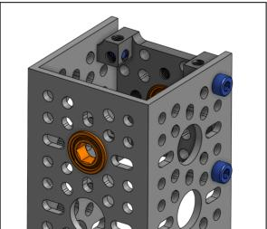
5. Fasten the 80mm REX axle to the flanged bearing in the Quad block. Use the mate connector on the REX axle for the connecting point.
