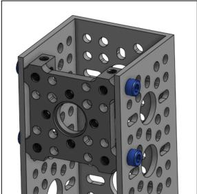
4. Attach the flanged bearings to the front and rear of the top portion of the 10 hole U channel with quad block:
