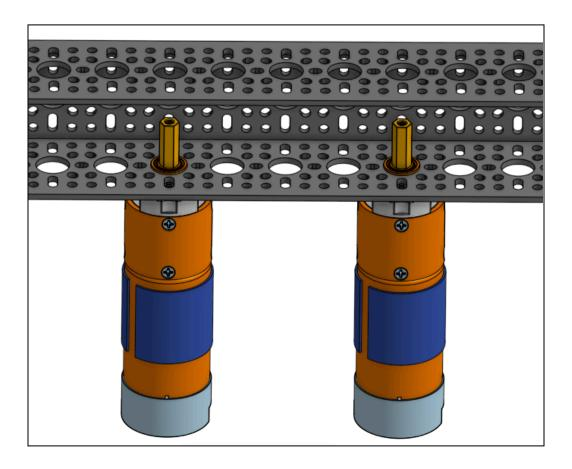
13. Attach the 8mm bolts (8x) to the two motors on the inside of the U Channel.
