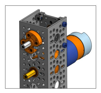
9. Use 4x 10mm bolts to bolt the motor to the U channel.
