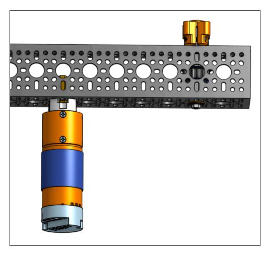
15. Repeat the process and attach the 2nd WheelAxle to the 2nd hole from the end of U Channel.
