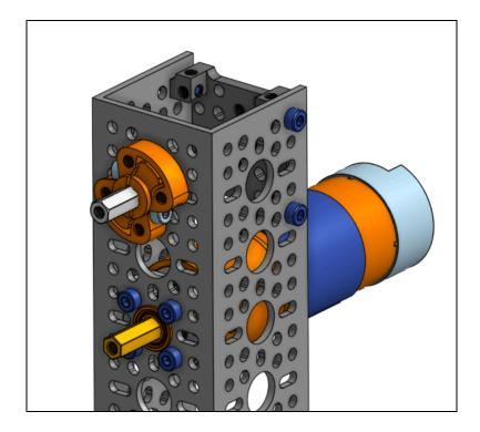
10. Attach the pinion gear to the motor shaft. Note the pinion gear is "reversed" on the axle with the narrow end facing out.
