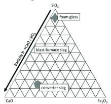
In this diagram you can see that this example converter slag has about 60% CaO, 25% iron oxides, and 15%  $SiO_2$ . Let's in our case assume 20% FeO and 5%  $P_2O_5$ , as well as 10% MgO substituting for CaO. MnO<sub>2</sub> often comes from the addition of manganese into the steel, which we don't do for simplicity.
