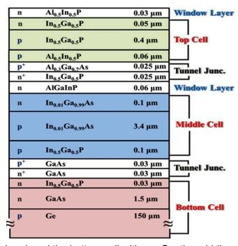
I replaced the bottom cell with p-n Ge, the middle cell base/emitter with GaAs, the middle window and tunnel junction layers with n-p AlGaAs. The ratios were simplified to 50-50 and an aluminium bottom and top contact layer as well as an ARC layer was added, patterned with PL.
