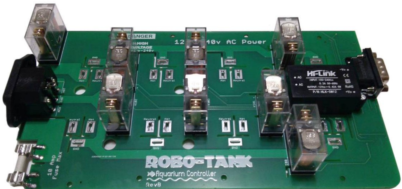
AC Power Bar Assembled
