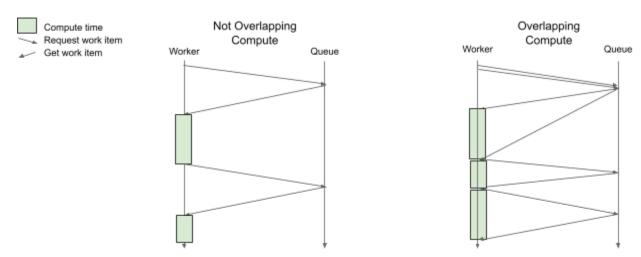
On the left we have the first code example where we synchronously call ray.get(get\_work\_item.remote()) to get a new work item to process. Because we have to wait for the RPC to return the next item, we have idle periods where we are not performing computation (represented as gaps in the green boxes).
