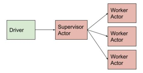
A single call to the supervisor actor triggers the dispatch of multiple method calls to child actors. The supervisor can process results or update child actors prior to returning.
