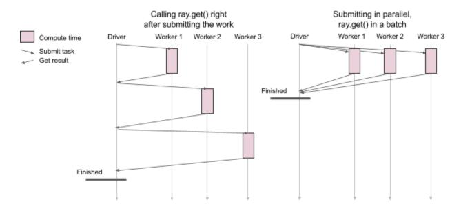
When calling ray.get() right after scheduling the remote work, the loop blocks until the item is received. We thus end up with sequential processing.
