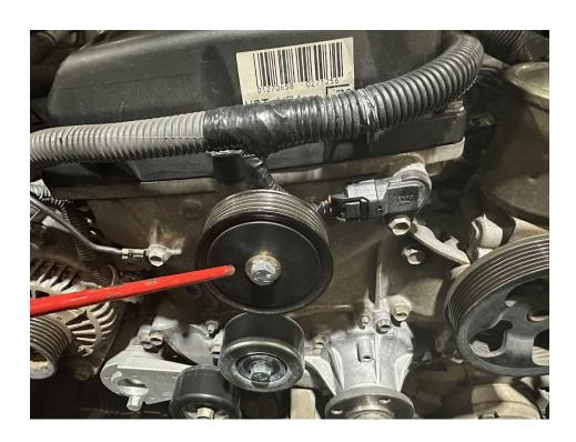
14.) Bend oil dipstick tube approximately 3" away from the steering pump to clear the charger and allow future access to the dipstick.
