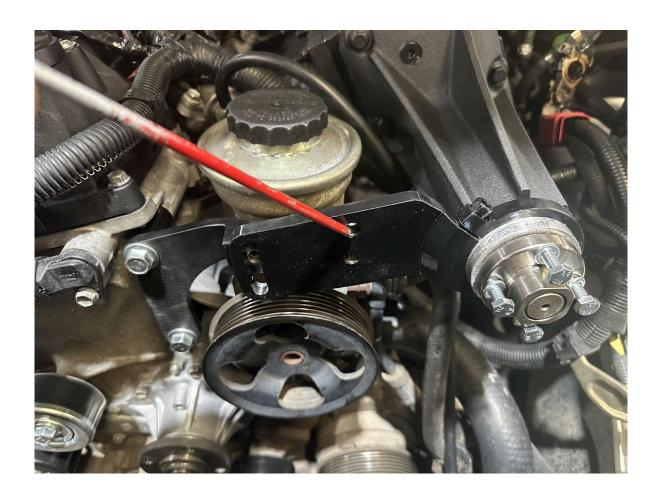
19.) Install tensioner to tensioner bracket 2 using supplied M10x60mm flange head bolt.
