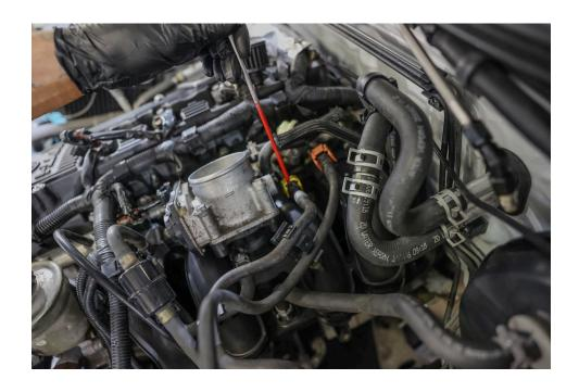
6.) Disconnect harness from EVAP VSV, remove bolt securing it to intake manifold and tie out of way. (See Image 3)
