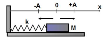
7. A block of mass M is attached to a horizontal spring k. The block undergoes SHM with amplitude of A. Which of the following graphs represents the kinetic energy as a function of position x?
