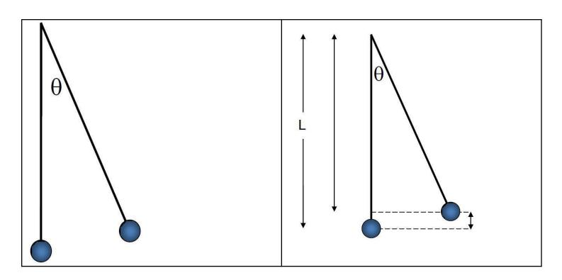
**Ex 1)** A pendulum is pulled back at an angle of 10. degrees from the vertical and is released. When the ball reaches the lowest point, it has a velocity of 2.0 m/s.
