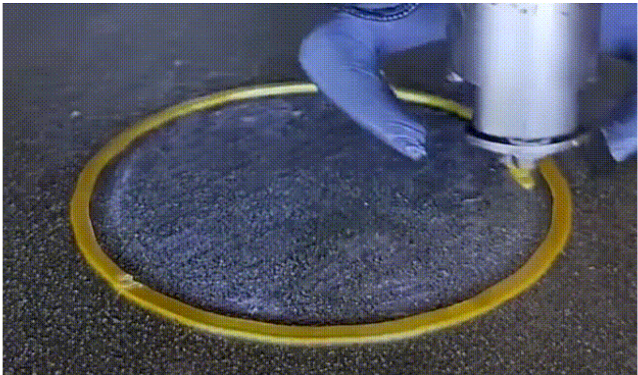
A Bondtech \text{Ø}1.8 mm CHT nozzle printing beads with a width of at least 2 mm wide.
