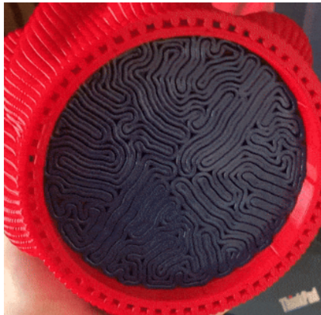
The unique look that a large nozzle can give to a print. Photo courtesy of Kowafatcompany
