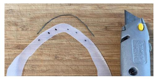
7. Thread the paperclip through the holes, use the needle nose pliers to pull or push the paperclip through the plastic. Start and end the paperclip threading, so that the ends of the paperclip are on what will become the outside of the mask (away from your face). That is, begin and end threading from the outside of the mask.
