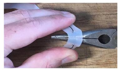
9. Create four small holes in the plastic (two on each side, above and below the mouth location), so that you can thread in strings. The holes can be made with the knife, or a hole punch if you have it.
