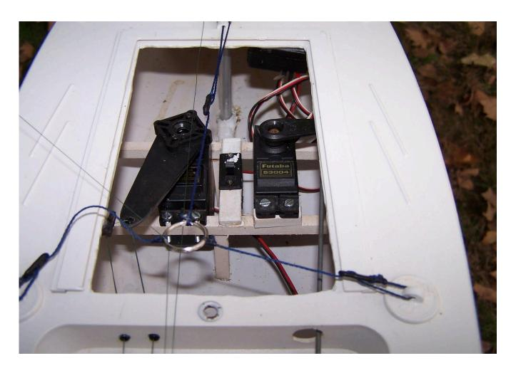
In the picture, the servos are mounted with the spline forward.
