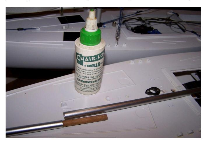
To CA plastic parts to the aluminum, I mask the tube with electrical tape and sand the area where the part should go with 80 grit sandpaper. Remove the tape. CA around the tube and slide the part into place.
