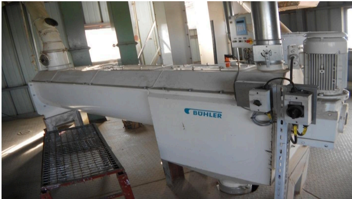
Fig 2.16 Malt polishing machine of Asella Malt Factory
