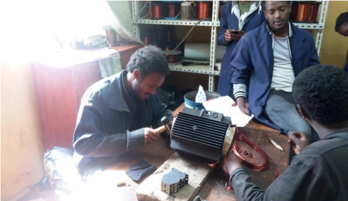
Fig.2.5 Concentric Winding of three phase induction motor
