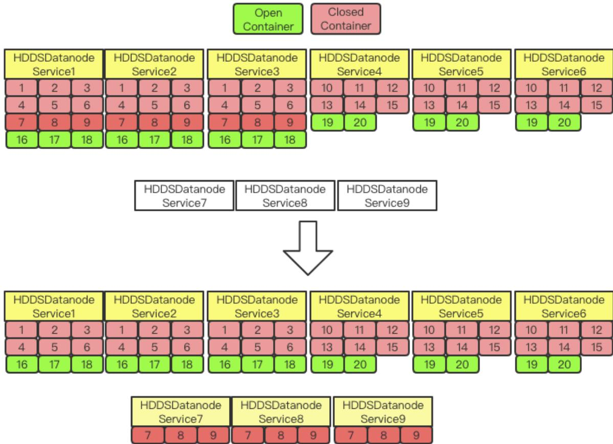
Let's say we have 6 existing datanodes in the current Ozone cluster, red block stand for closed container, green block stand for open container, the number in the block means the container id.
